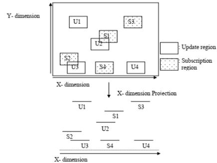
**Figure 2: Dimension Projection with the X Dimension**
